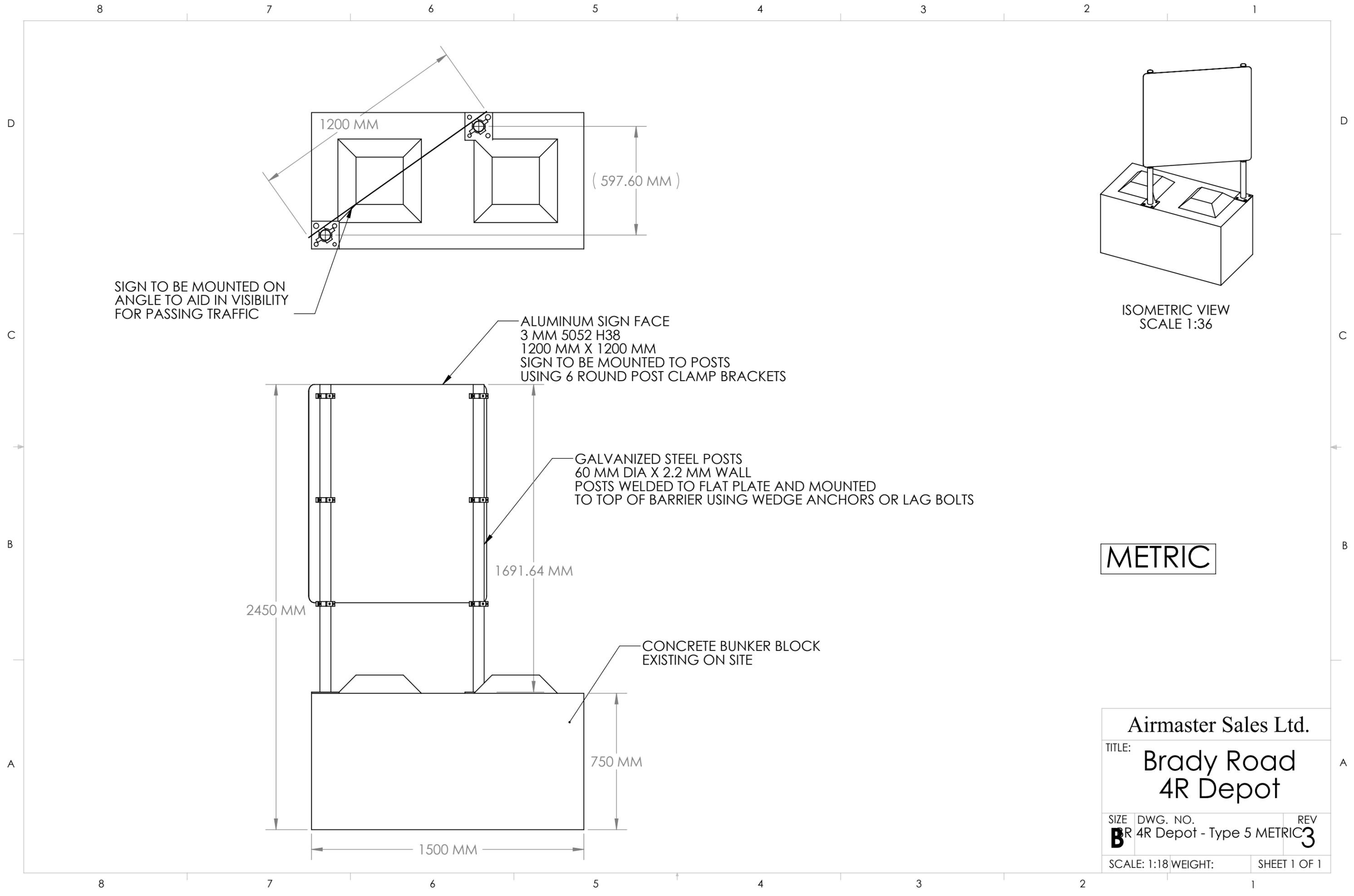
SIGN TO BE MOUNTED ON ANGLE TO AID IN VISIBILITY FOR PASSING TRAFFIC
